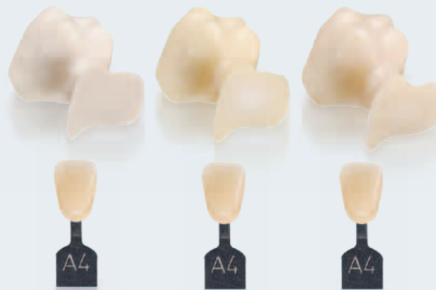
Sliced pontic of monolithic zirconia 3-unit bridges, A4 shaded according to instructions for use of manufacturer. From Left to Right: Crystal™ HS, VITA In-Ceram® YZ, Lava™ Plus High Translucency Zirconia.
