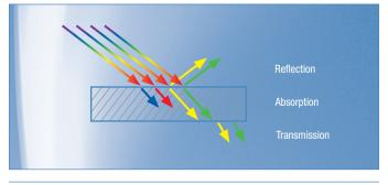
fig. 2 Example of reflected an transmitted light versus absorbed light. The observer detects light of the remaining wavelength, in this case green and yellow light.
