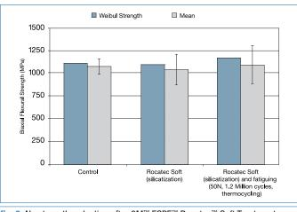
fig. 3 No strength reduction after 3M<sup>™</sup> ESPE<sup>™</sup> Rocatec<sup>™</sup> Soft Treatment (30µm) of 3M<sup>™</sup> ESPE<sup>™</sup> Lava<sup>™</sup> Zirconia initially and after cyclic loading and thermocycling (50N, 1.2 Million cycles).
