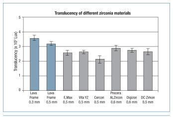
fig. 2 Light intensity transmitted through zirconia copings as detected by photo-radiometer
