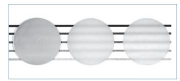
fig. 7 Translucency of platelets of Lava<sup>™</sup> Zirconia depending on the thickness of the material (Courtesy, Prof. Dr. D. Edelhoff, University of Munich).
