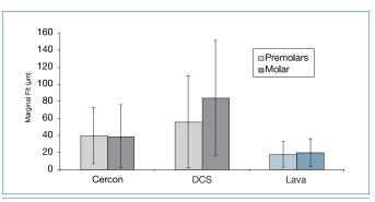
fig. 2a Marginal gap of 4-unit zirconia 3M<sup>™</sup> ESPE<sup>™</sup> Lava<sup>™</sup> Bridges in comparison to competitor systems. A. Piwowarczyle and H.C. Lauer, University of Frankfort.<sup>2</sup>
