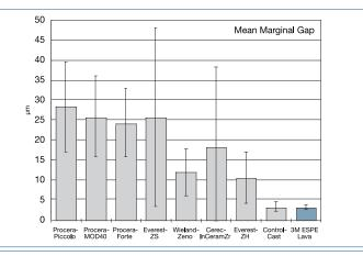
fig. 4 Vertical marginal gap of 3M<sup>™</sup> ESPE<sup>™</sup> Lava<sup>™</sup> Copings in comparison to competitor systems. A.J.T. Shannon et al., University of Iowa.4
